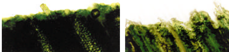
Grass Blade Tips magnified x 75 Non lapped cut – left : Lapped mower cut - Right
